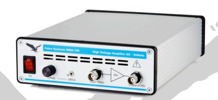
The WMA-100 is a compact all-round, general-purpose high voltage linear amplifier. It offers a wide output voltage range (±175V), DC offset control, and impressive bandwidth (DC - 500kHz) and noise (350  $\mu V_{rms})$  specifications. The amplifier generates no overshoot with any capacitive load. The short-circuit protection with a fast current limit make this amplifier suitable for both normal daily laboratory use and automated measurement systems.
